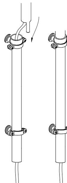
Pull precisely and with caution at the power cord to ensure a tight fitting of the two lamp parts
